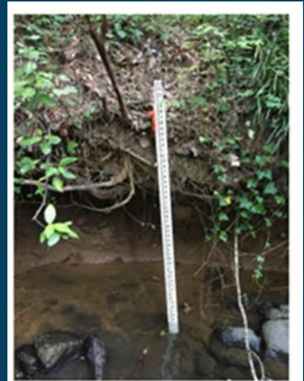
BP #2 — UT to Ellerbe Creek BEHI: High | NBS: Very High Location: Museum of Life and Science
