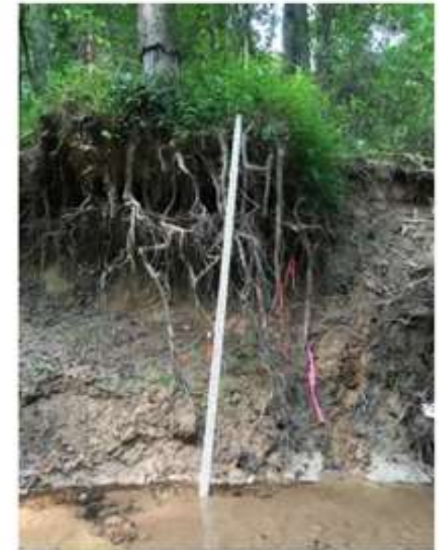
BP #1 — UT to Ellerbe Creek BEHI: Extreme | NBS: Extreme Location: Camden Ave.
