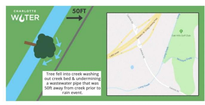
Depiction of how creek flow washed away the soil around a sewer pipe, causing it to collapse and spill.
